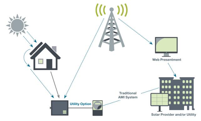
How it Works Smart Meter communication over cellular networks
