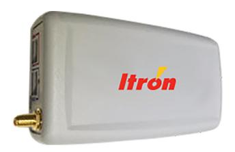
A portable field device that uses RF to communicate with network devices such as meters or Distribution Automation (DA) devices. The FSU can perform a full range of RF configuration and network diagnostic tests, including register reads and firmware upgrades.
